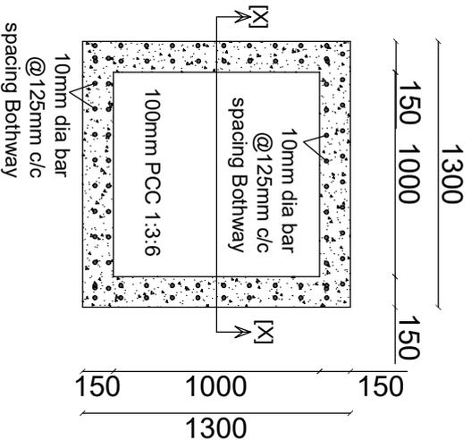
Intermediate Tank Reinforcement Detail
