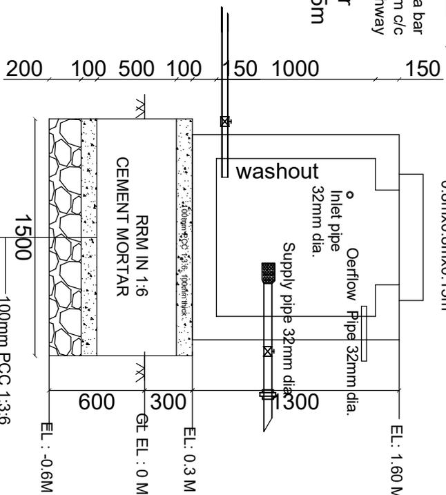
Intermediated Tank Section at [X]-[X]
