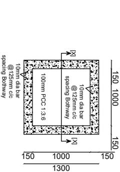
Intermediate Tank Reinforcement Detail
